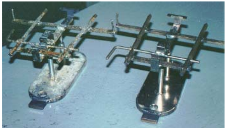
Headlamp carriers before and after cleaning.
